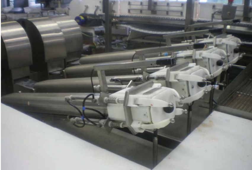
Figure 2.14. Pi-Vac Elasto Pack System® equipped for four different packaging sizes.
