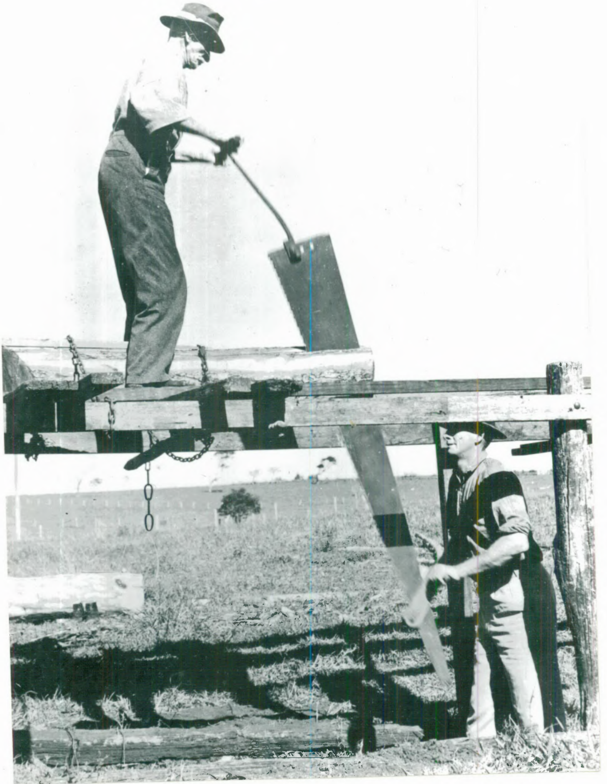
PIT-SAWING : George Vidler (b.1874) and his son John demonstrating pit-sawing on a scaffold saw-pit on H.M. Crawford's property at Tregeagle in 1956. The saw which had belonged to his father, had been in George Vidler's possession for 65 years at this time. Photo : RRHS, originally published in The Northern Star , 28 June 1956.
