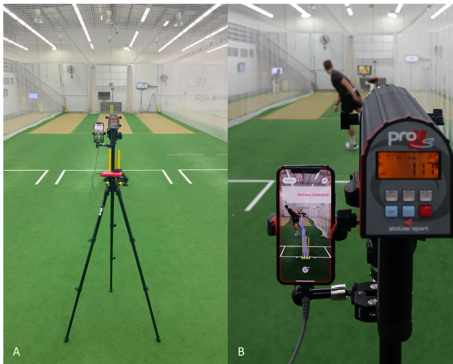
Figure 1. Testing set-up: A: position of the Stalker Pro IIs radar gun and iPhone running the Fulltrack AI application relative to the wicket B: zoomed in perspective view of each device.
