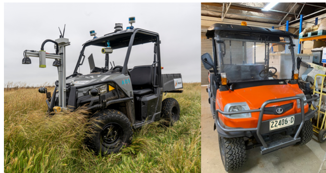
FIGURE 1.2: The two vehicles used for image capture in this study. On the left is the Polaris Ranger EV, showing the data collection rig. On the right is the Kubota RTV 900XT.
