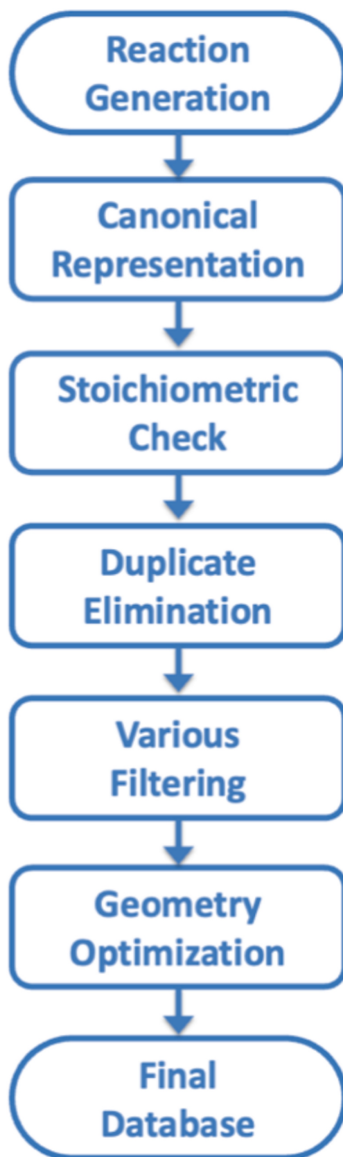
Fig. 1. Schematic representation of the automated workflow for generating chemical reaction databases.
