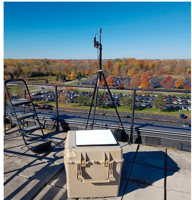
Fig. 1. The OpenHSI hyperspectral imager scans the sky from a tripod and rotation stage. We set up the camera and Spectralon™ panel on the roof to minimise occlusions.
